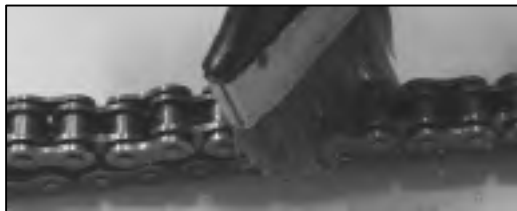
Cleaning and coating with oil
