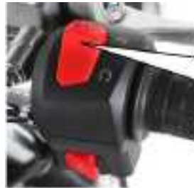
Emergency "Kill" Switch
