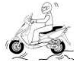
TIRE PRESSURE TOO LOW
