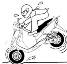
TIRE PRESSURE TOO HIGH
