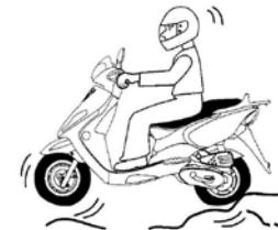
TIRE PRESSURE TOO LOW
