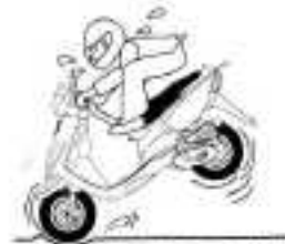
TIRE PRESSURE TOO HIGH
